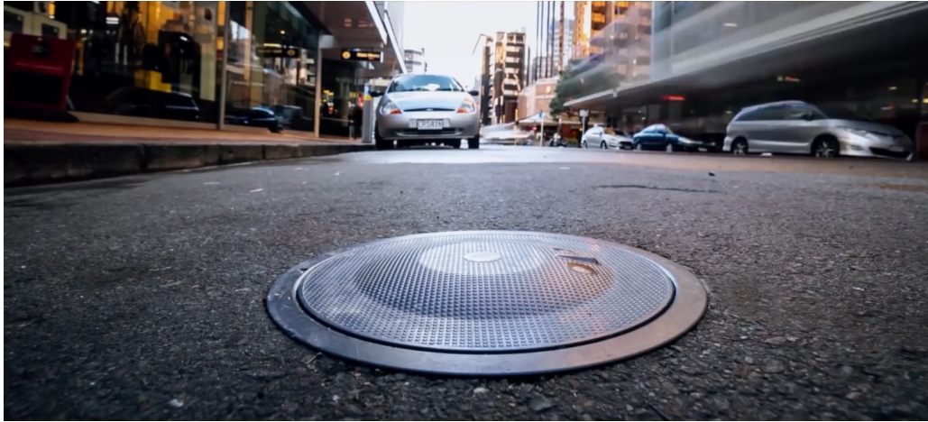
Figure 5: Example of ground sensor for detecting parking spot occupancy. (source: https://www.asmag.com )
