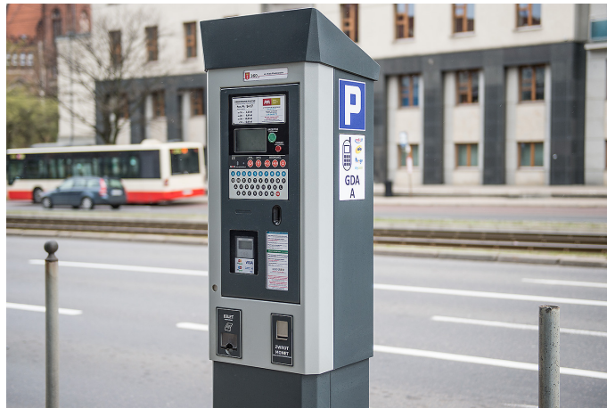
Figure 1: Parking meter in the city of Gdańsk. Accepts payment by cash or card. When license plate number is provided, there is no need to put the ticket under the front window of the car (source: https://www.trojmiasto.pl/ ).
